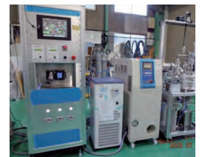
Friction and wear test equipment in a hydrogen atmosphere
